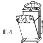
3. Close the Front Pressing Plate and carefully pull the Pressing Bar back down far enough so that it holds the Front Pressing Plate closed. Do not pull the Pressing Bar all of the way down. Do not lock it into place yet. 4
