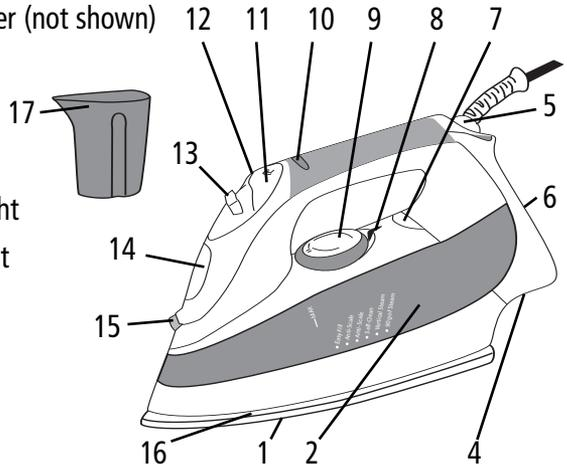
1. **Profiled Soleplate** – Maximum glide, durable ceramic soleplate with **Preconditioning Steam Vents**, allow steam to reach the fabric before the heated soleplate.
