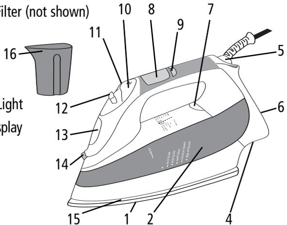
1. **Profiled Soleplate** – Scratch resistant stainless steel soleplate with 'Leading Edge' steam outlets that channel steam to the soleplate tip.
