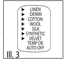
After 3 seconds the Velvet setting (lowest setting) will flash in the display window. Press the '+' Temperature Control Button to increase the temperature. The selected fabric will flash until the soleplate has reached the selected setting. The Iron will beep and 'TEMP OK' will appear in the display window when the iron is at the selected setting.
