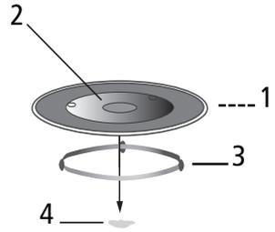
Center the Turntable Ring over the Turntable Shaft on the floor of the microwave oven. Install the Glass Tray, centering the Hub over the Turntable Shaft. Turn the Glass Tray slowly until the Hub engages on the Turntable Shaft.
