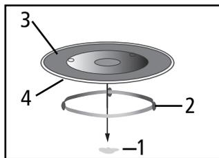
Center the Roller Ring over the Turntable Shaft on the floor of the Microwave. Install the Glass Tray, centering the Hub over the Turntable Shaft. Turn the Glass Tray slowly until the Hub engages on the Turntable Shaft.
